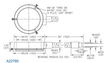
Warning: This product is manufactured with glass fiber. Not for use in cable/hose carrier. Call SCHOTT to discuss moving cable/hose carrier applications.
